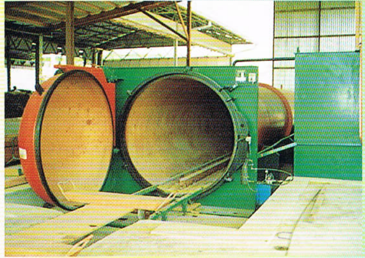
DWT T10 impregnation plant for impregnation of timber with water-borne wood preservatives
