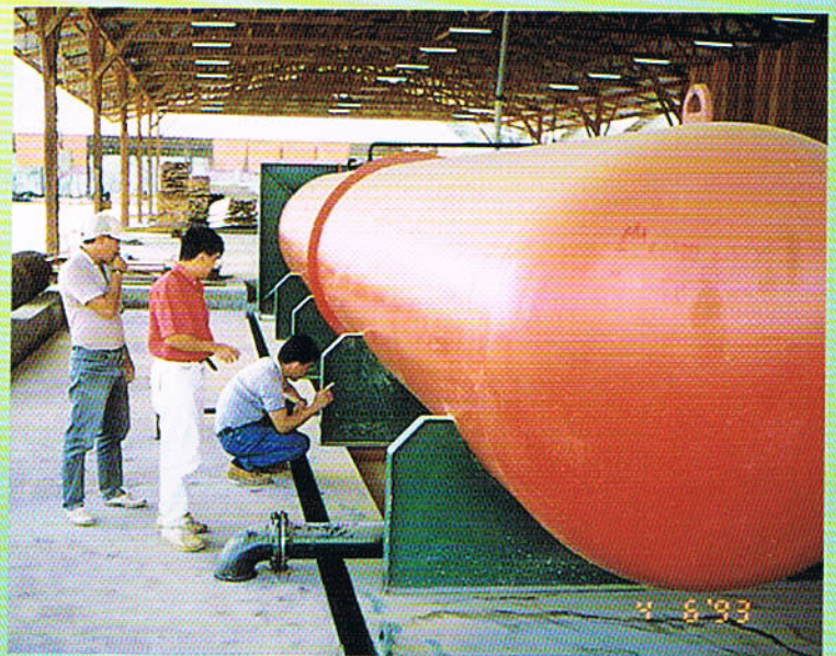
The DWT T10 impregnation plant is supplied with up to two storage tanks installed below the pressure vessel.
