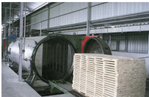
A lumber charge getting ready for the Hydro-Thermo treatment Process
