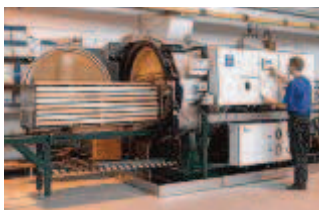
A completed load of treated hardwoods ready to exit the treatment vessel
